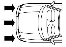
frontal and near-frontal collisions, not rollover, side-impact, or rear-impacts unless the collision causes sufficient longitudinal deceleration.
